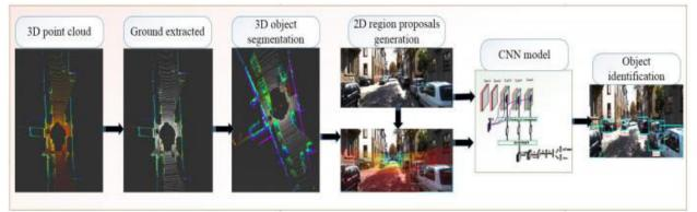
Figure2. The suggested framework for the multi-object detection method is described in detail.
